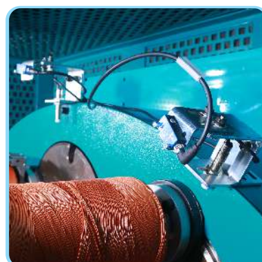
Bobbin empty and Wire cut sensors
