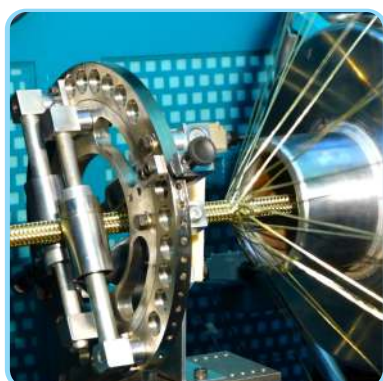
Adjustable guide rollers for different hose diameters
