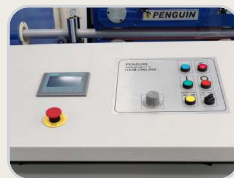
Control panel with HMI
