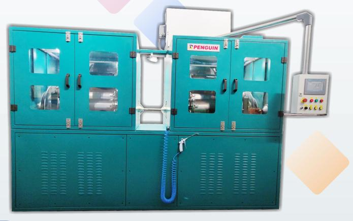
construction of spiral structure of yarn over rubber hose. Spiraling is done to increase the strength of rubber hose. The spiraled rubber hose can be used in production of low and medium pressure hoses.
