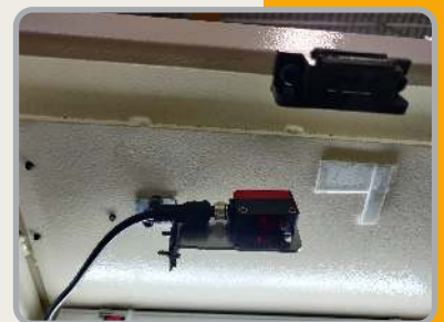
Photo sensor stop motion for yarn cut
