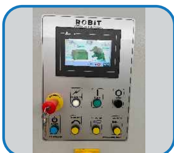
Push button station with PLC
